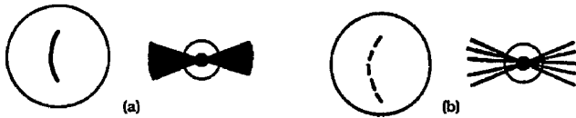
Fig. 14. Curved spider producing two searchlight beams emanating in opposite directions from the image core. This is intuitive if one approximates the curve as a set of straight segments.
